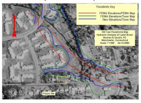
As part of a residential site plan, Meehan & Goodin prepared a detailed hydraulic analysis to delineate the 100 year floodplain for a section of **Lydall Brook** in **Manchester**, CT. Aerial photographs aided in the presentation of the results of this analysis.
