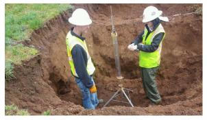
When Gengras Volvo planned to construct a new dealership in North Haven, they returned to Meehan & Goodin to prepare the land surveys, site plans, and permit assistance that would be required. Shown above is a field hydraulic conductivity test being performed by GEI Consultants as part of our storm drainage design
